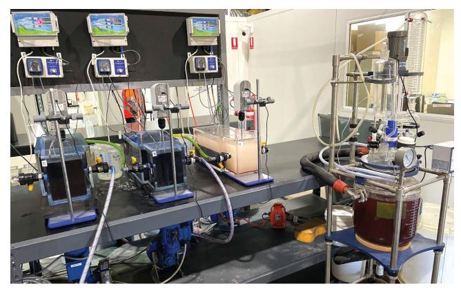
Figure 4 – Solvent extraction and cobalt sulphate crystalliser
