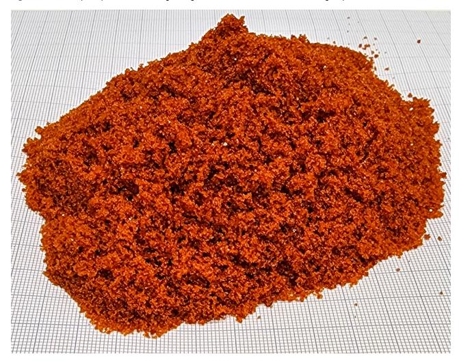
Figure 6 – Refinery Project – Cobalt Sulphate produced from commercial third-party feedstock
