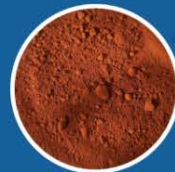
Leach Residue Fe 2 O 3
