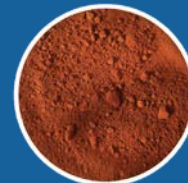
Leach Residue Fe 2 O 3
