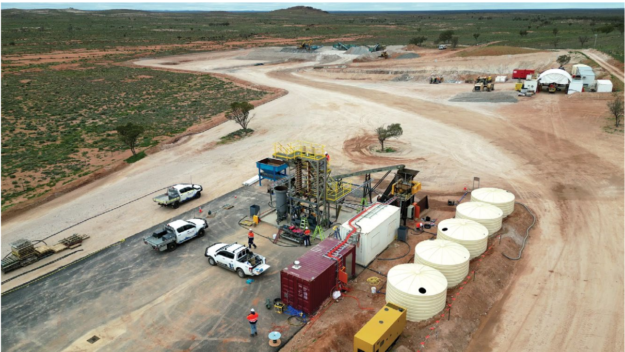
Figure 5 – Pyrite Hill site concentrator including gravity spirals.
