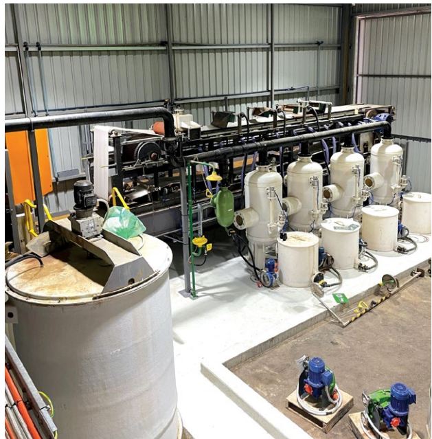
Figure 2 – Broken Hill plant. Left: Iron oxidation and precipitation circuit. Right: Installation of iron polishing and MHP precipitation circuits.
