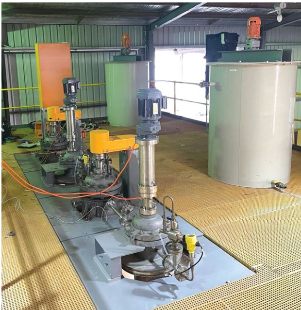
Figure 2 – Broken Hill plant. Left: Iron oxidation and precipitation circuit. Right: Installation of iron polishing and MHP precipitation circuits.
