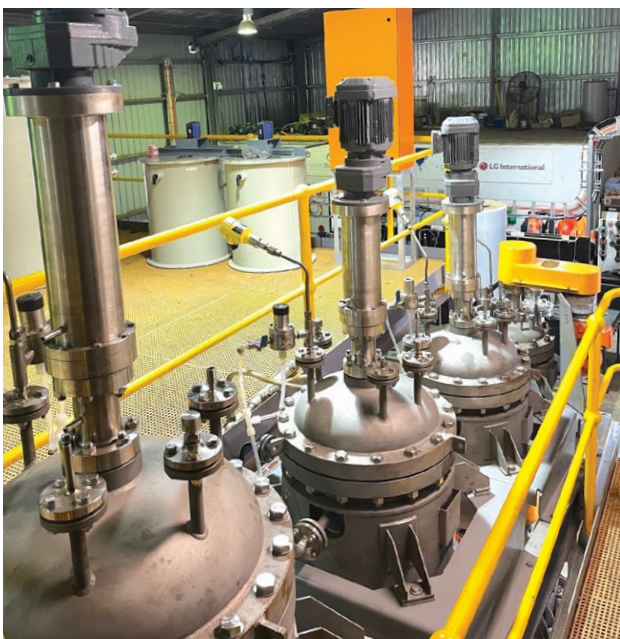
Figure 2 – Broken Hill plant. Left: Iron oxidation and precipitation circuit. Right: Installation of iron polishing and MHP precipitation circuits.
