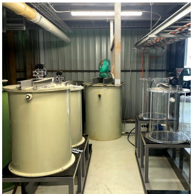
Figure 2 – Broken Hill plant. Left: Iron oxidation and precipitation circuit. Right: Installation of iron polishing and MHP precipitation circuits.
