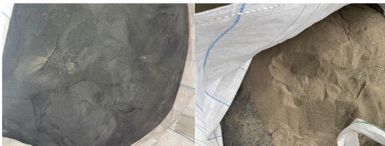
Figure 6 – Kiln product separated into pyrrhotite for leaching (left hand side) and gangue (right hand side) for recycle to the float cell for recovery of unreacted pyrite.
