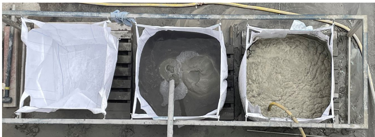
Figure 2 – Collection of concentrate into 1 tonne bulka bags with float concentrate on the left, and gravity concentrate in the centre
