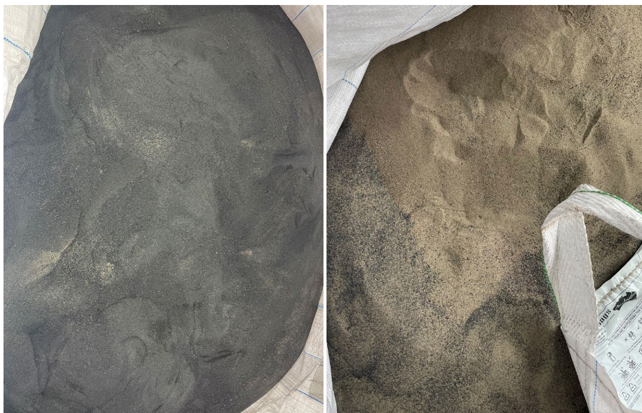
Figure 5 – Kiln product separated into pyrrhotite for leaching (left hand side) and gangue (right hand side) for recycle to the float cell for recovery of unreacted pyrite.
