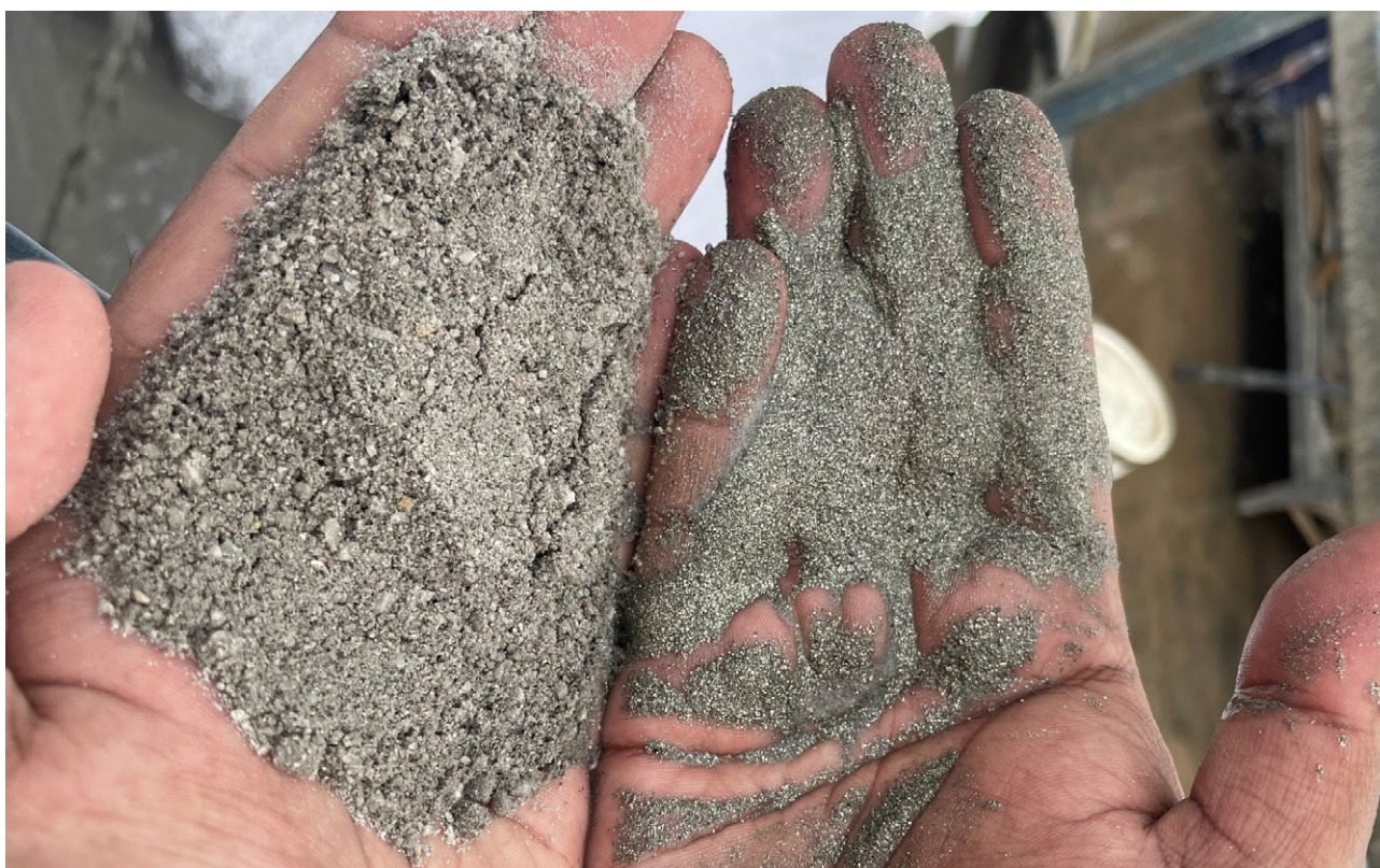
Figure 4 – Feed ore milled to <4 mm on left hand, and gravity concentrate on right hand
