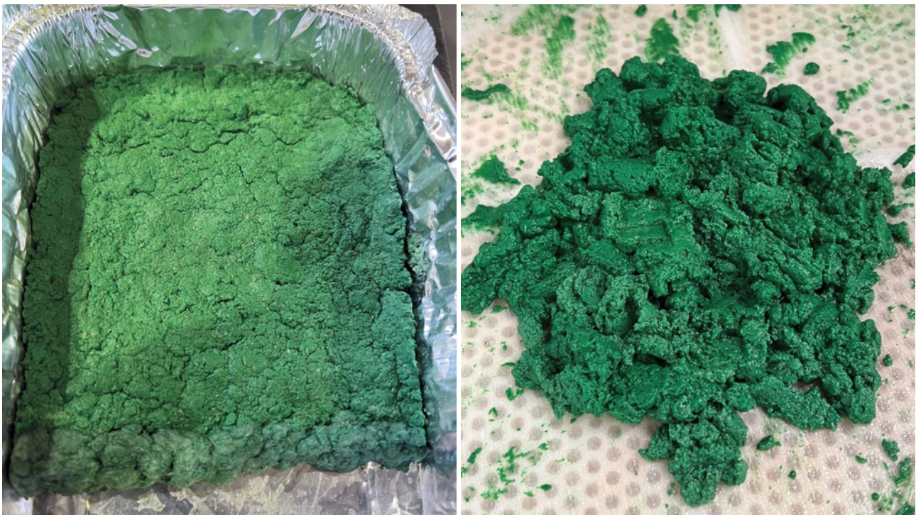
Figure 6 – First batches of Mixed Hydroxide Precipitate (MHP) from the BHCP Demonstration Plant
