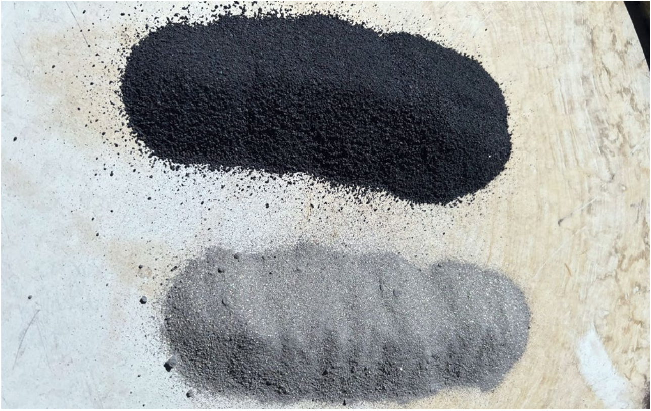
Figure 4 – Elemental sulphur produced from the calcining of concentrate in the kiln.
