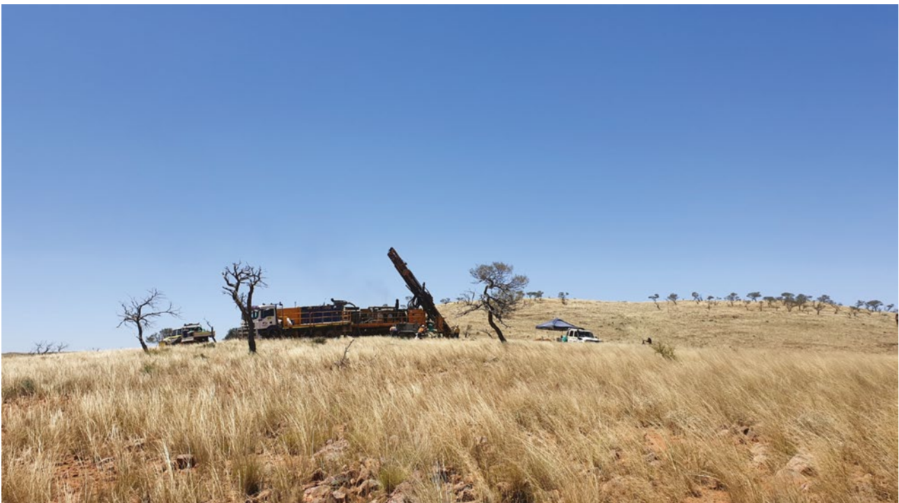
Figure 7 – Reverse circulation drilling operations.
