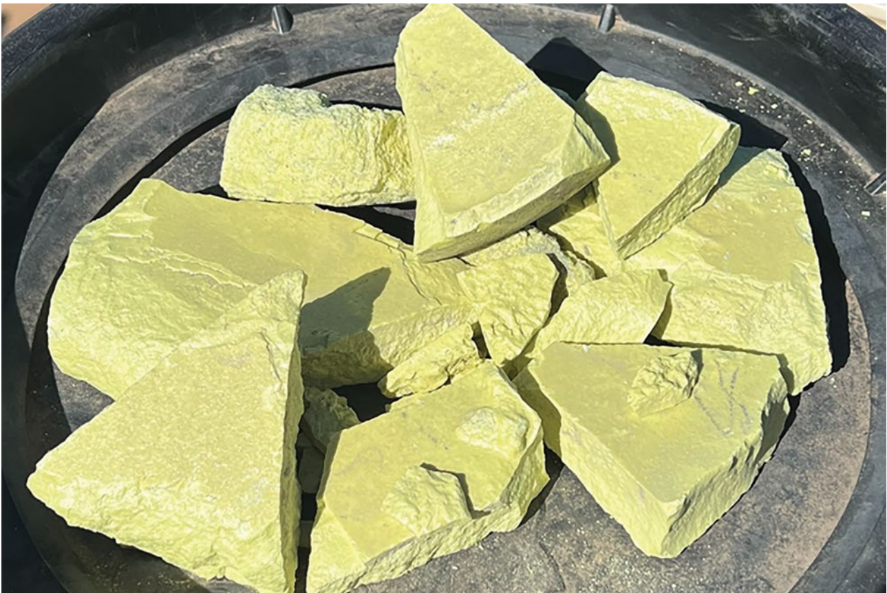
Figure 4 – Elemental sulphur produced from the calcining of concentrate in the kiln.
