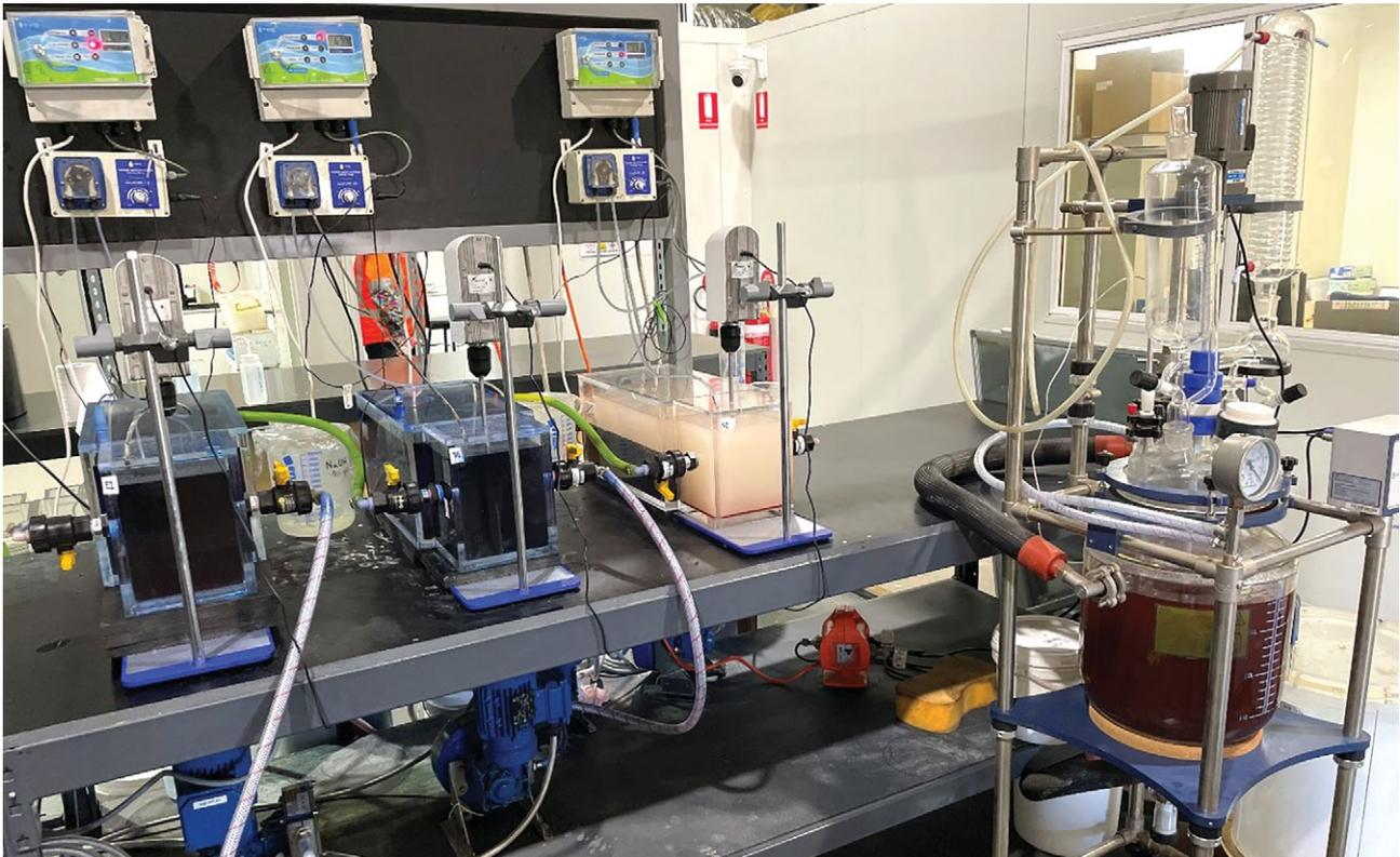
Figure 5 – Cobalt solvent extraction strip cell
