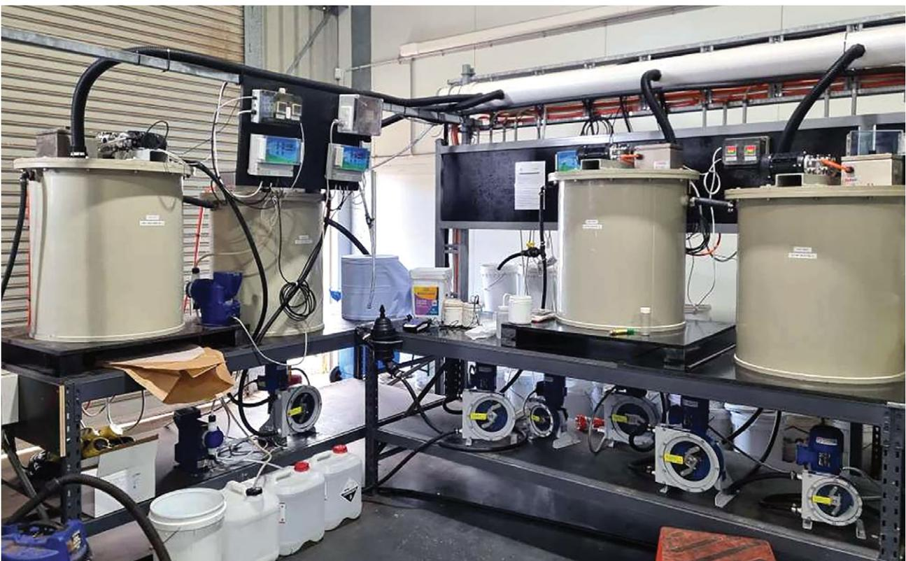
Figure 4 – Solvent extraction and cobalt sulphate crystalliser
