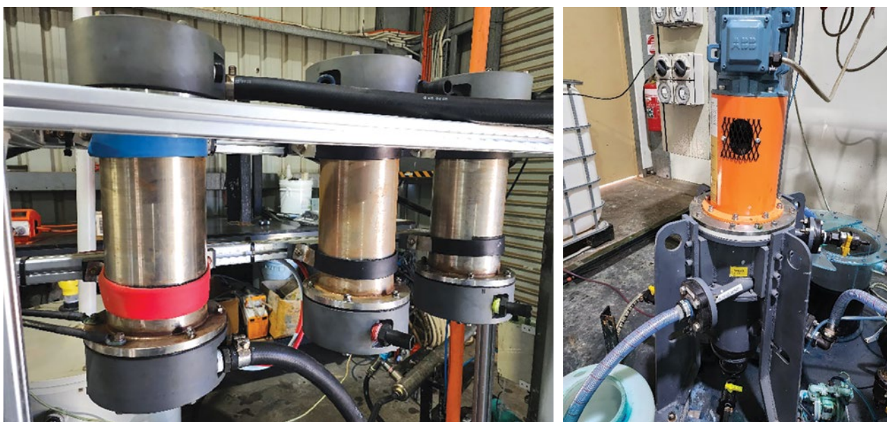
Figure 1 – Electrowinning cells used for testing (LHS) and Centrifugal extractor (RHS)
