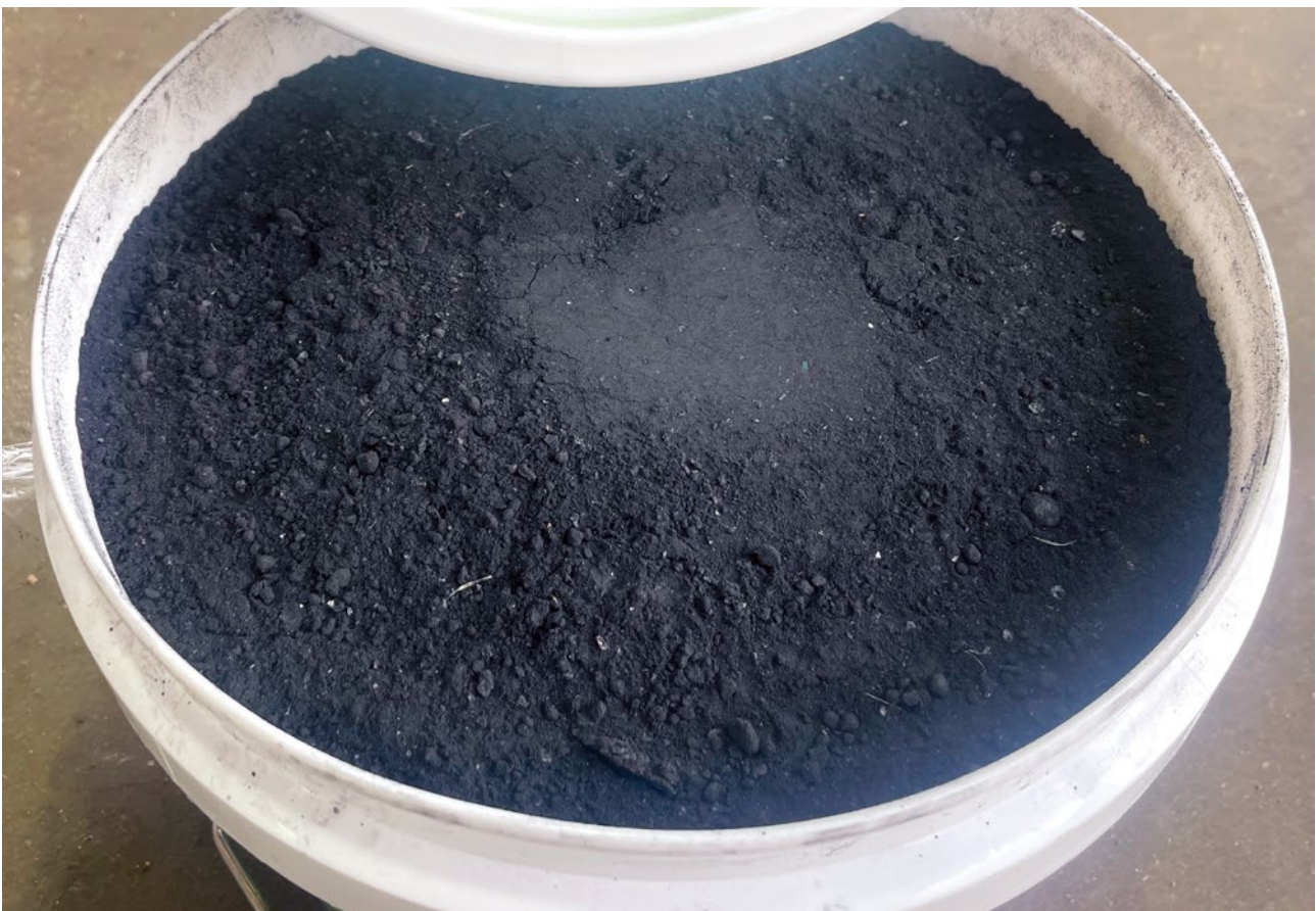
Figure 4 – Ecobatt's black mass ahead of testing at the Broken Hill Technology Development Centre
