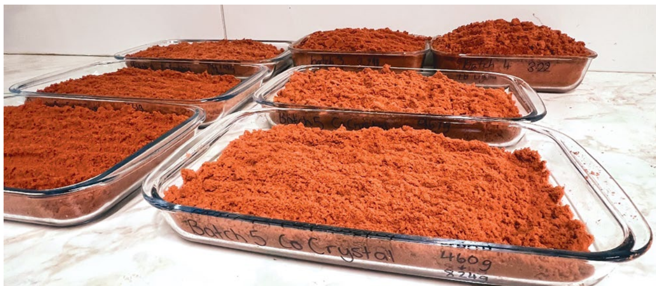
Figure 2 – Cobalt sulphate produced at the Broken Hill Technology Development Centre Plant
