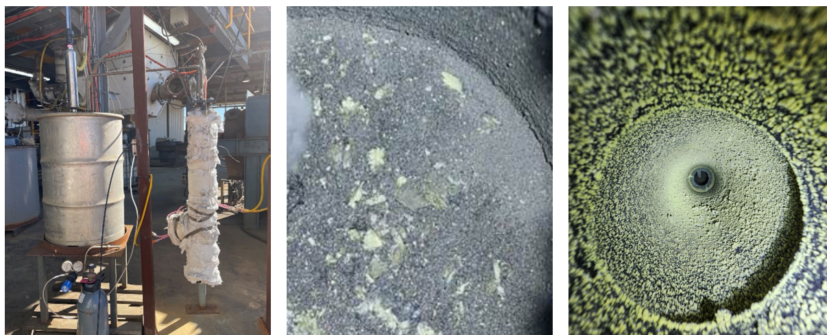
Figure 4 - (L-R) Vertical kiln prototypes, pyrrhotite product after pyrite conversion and sulphur collection in condenser.
