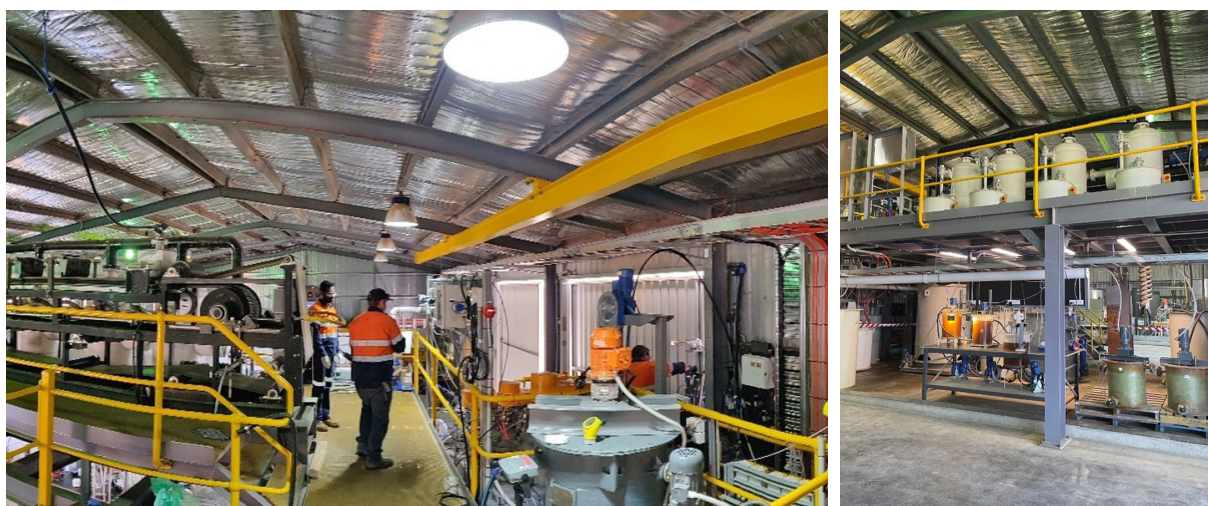
Figure 3 - Pressure oxidation and iron precipitation circuits at the Broken Hill Technology Centre.
