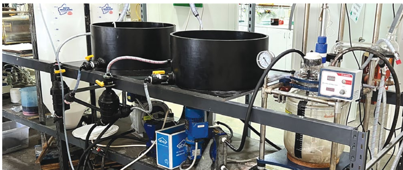
Figure 1 – Cobalt sulphate crystalliser and filtration pans
