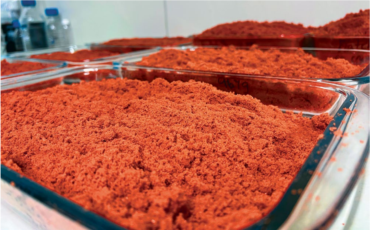
Figure 2 – Cobalt Sulphate crystals produced from third party feedstocks
