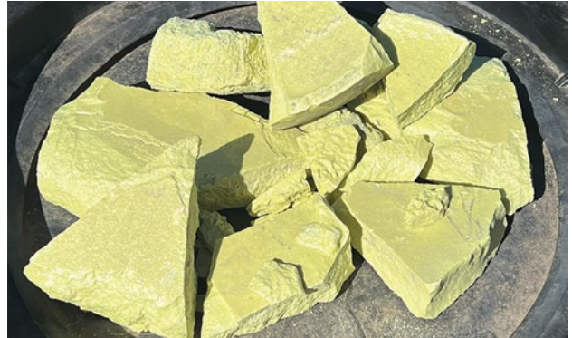
Figure 9 – Mixed hydroxide precipitate containing both cobalt and nickel, produced from cobaltiferous pyrite.
