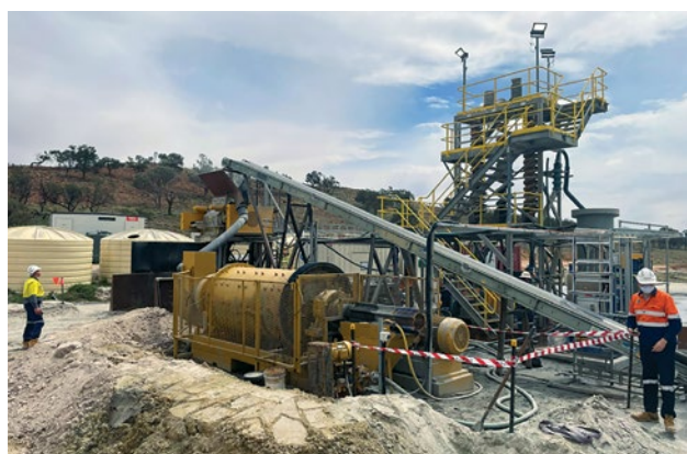
Figure 4 – Demonstration plant, comminution circuit.
