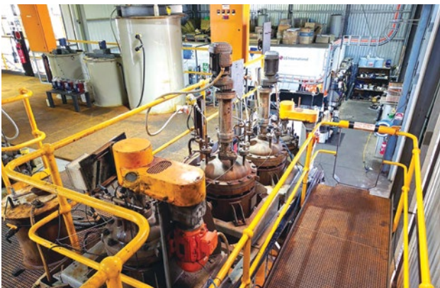
Figure 8 – Demonstration plant, pressure oxidation circuit.
