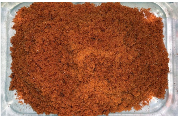
Figure 10 – Battery grade cobalt sulphate produced from cobalt bearing pyrite.
