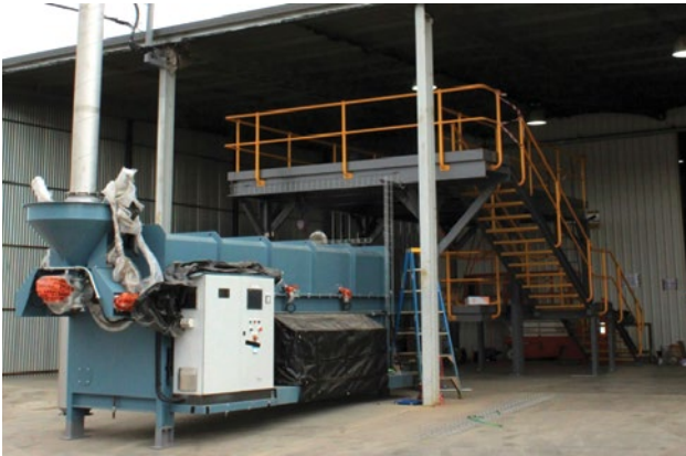
Figure 6 – Demonstration plant kiln.
