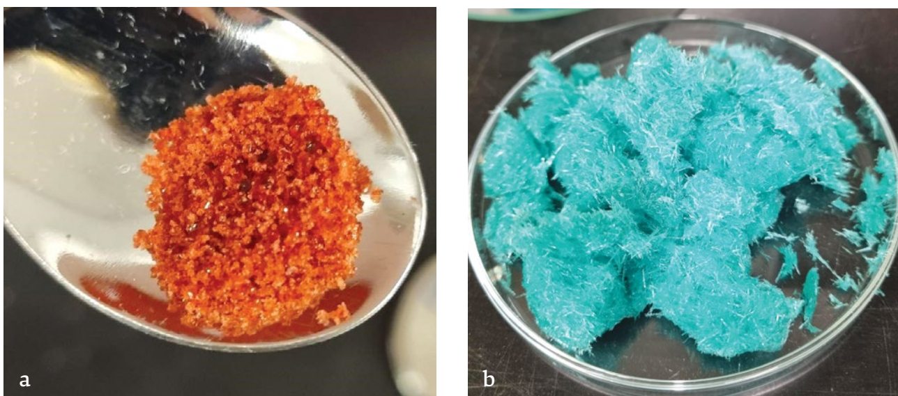
Figure 3 – Cobalt and nickel sulphate crystals produced in development testwork
