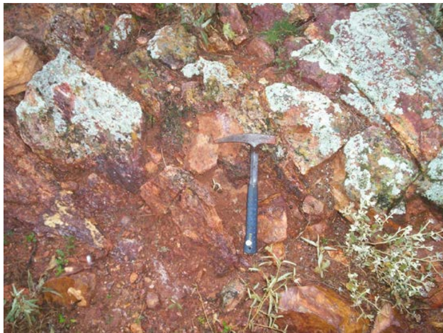
Photo 1: Highly gossanous (60% pyritic boxworks) band in quartz albitic rock
