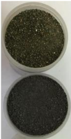
Figure 44: Pyrite feed and calcined pyrrhotite
