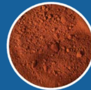
Leach Residue Fe 2 O 3
