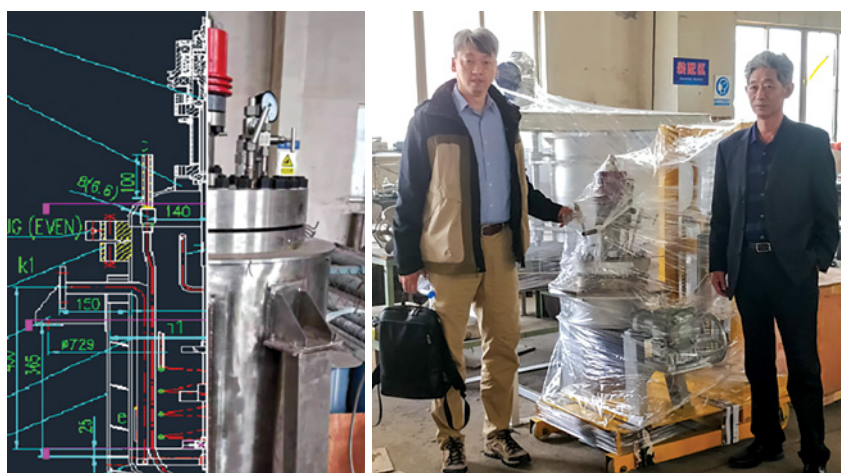
Figure 3. Design drawing and cutaway of leach reactor (LHS), fully assembled similar reactor on factory floor (RHS).
