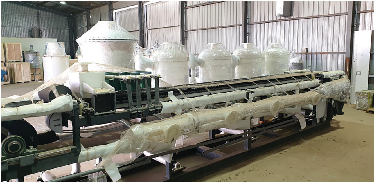
Figure 2 – COB Pilot Plant – Vacuum Belt Filter and Reactors (foreground)
