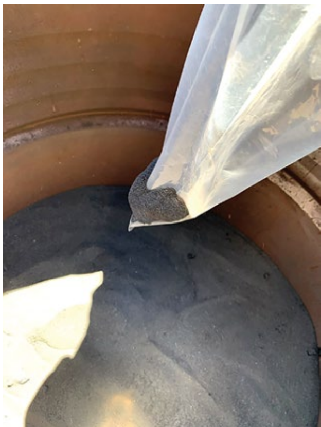
Figure 3 – Calcined product – Pyrrhotite
