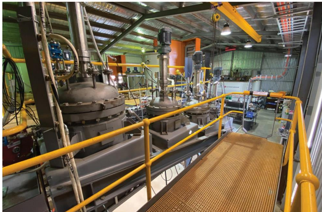
Figure 26: Demo plant pressure oxidization leach circuit
