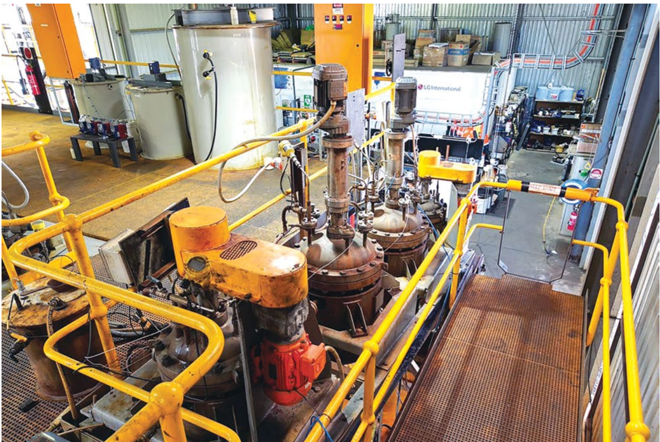
Figure 7 – Pressure oxidation leach circuit
