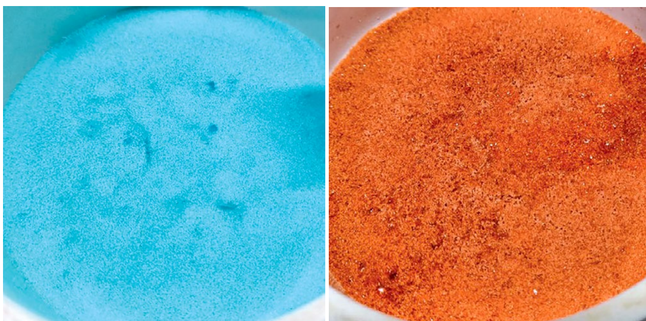
Figure 2 – Demonstration Plant – nickel sulphate and cobalt sulphate
