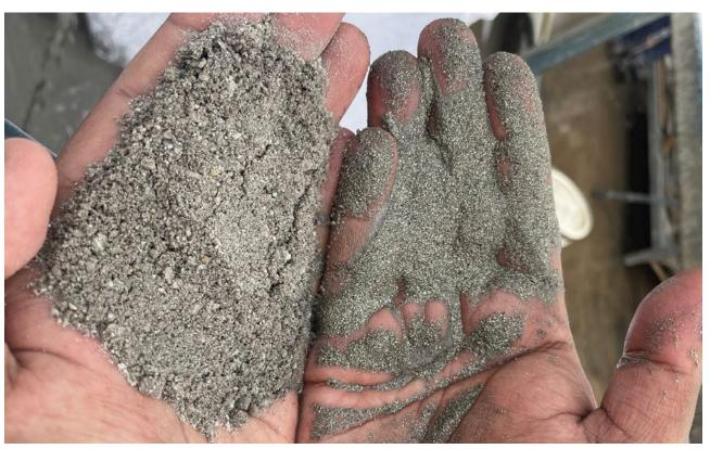
A total of 4,200t of ore was processed to produce 680t of wet concentrate (typical moisture 5–10%). A further 800–1,000t of ore remains for optimisation studies in the future. Operations were held over 65 days with the longest run of over 100 hours recorded. Mass recovery of ~17–20% was consistently achieved, with an average concentrate grade of 4,434 ppm Co (see Figure 6).
