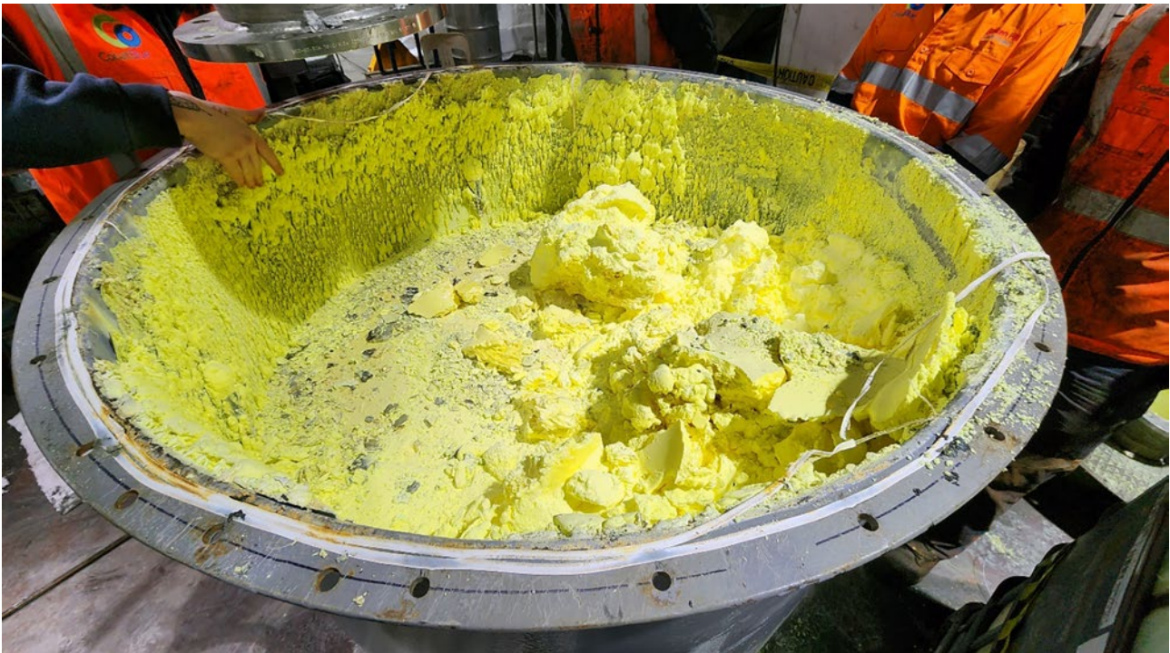
Figure 2 – Sulphur in the condensation tank and after emptied from the tank
