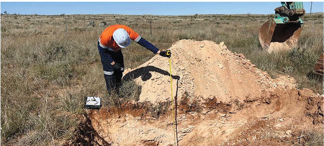
Figure 5 – Geotechnical consultant logging a shallow test pit at the intersection of the proposed access road and Barrier Highway
