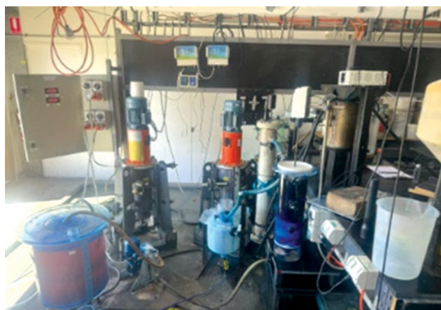
Figure 4 – BHTC's cobalt solvent extraction circuit
