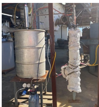
Figure 2 – (L–R) Vertical kiln prototypes, pyrrhotite product after pyrite conversion and sulphur collection in condenser
