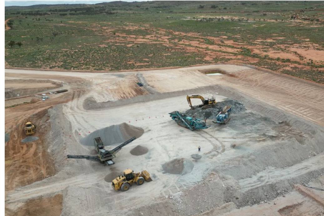
Ore primary crushing in progress. ROM ore is crushed through jaw crusher to <75mm, then cone crusher to <22mm. That is then screened over a 4.5mm screen.
