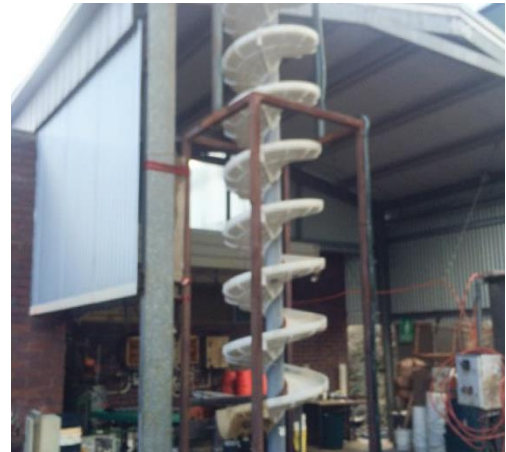
Concentrate testwork – simple gravity spirals delivering exceptional results
