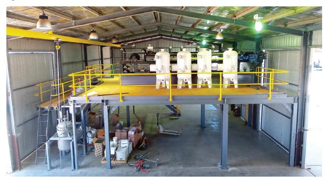
Figure 2 – Pilot Plant – installed autoclave reactors in foreground
